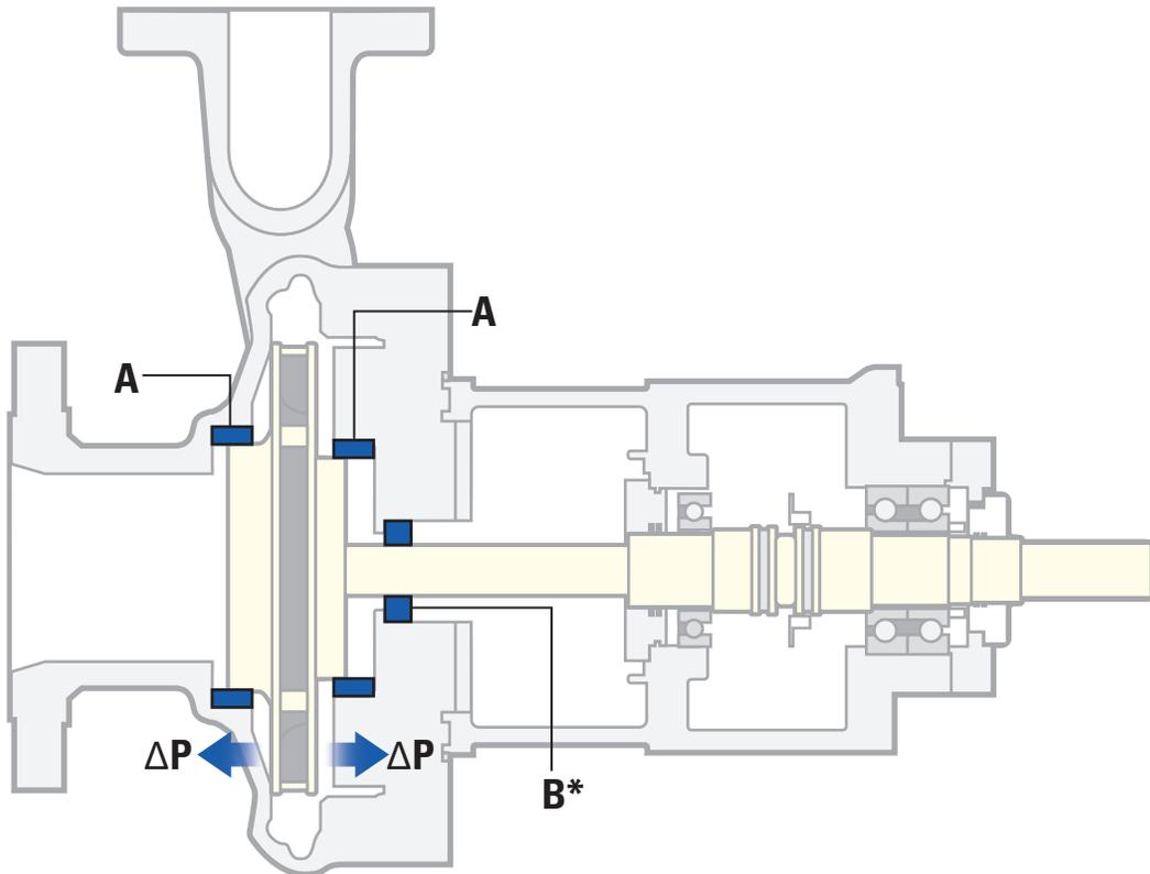
**A.** Case Wear Rings **B.** Throat Bushings  $\Delta P$ . Direction of differential pressure
