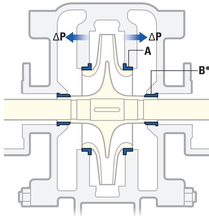
**A.** Case Wear Rings **B.** Throat Bushings  $\Delta P$ . Direction of differential Pressure
