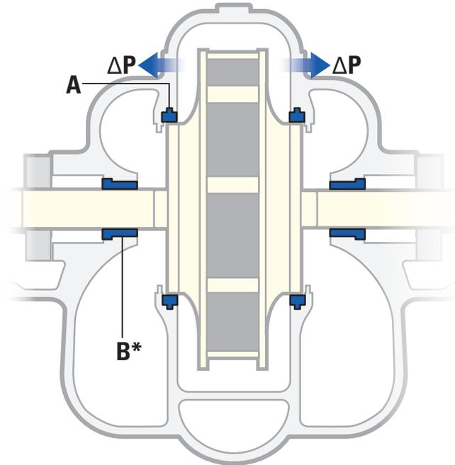
**A.** Case Wear Rings **B.** Throat Bushings  $\Delta P$ . Direction of differential pressure
