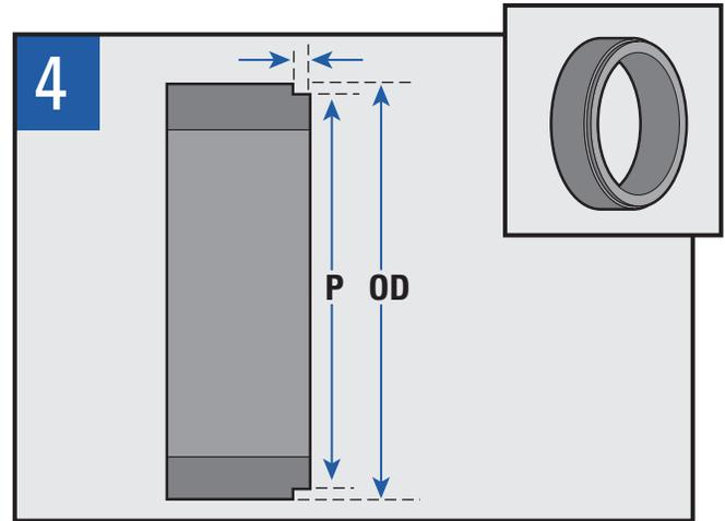
Machine the leading edge with pilot fit.
