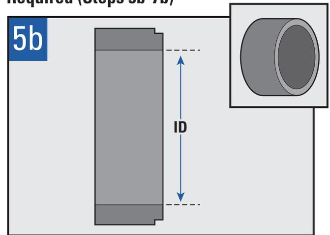
Calculate and machine part inside diameter.
