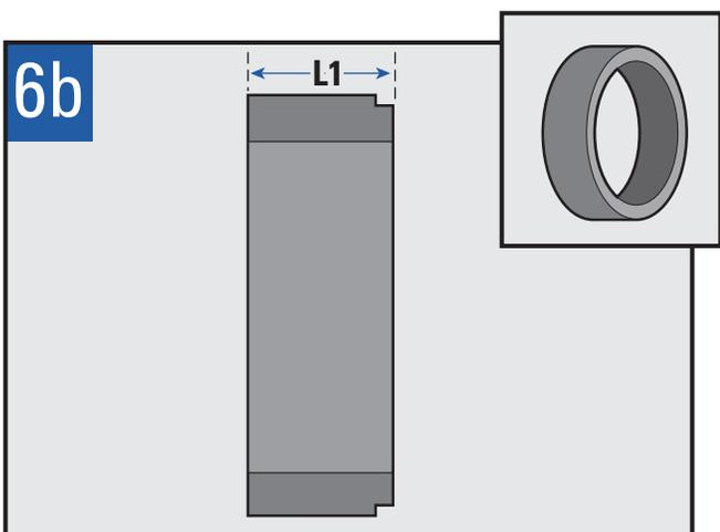
Calculate and machine part **L1** (overall part length).
