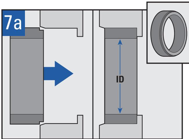
Press into place, final machine inside diameter
