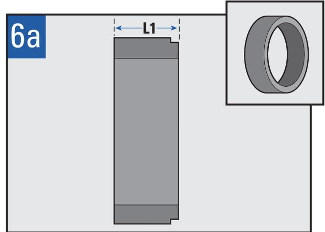
Calculate and machine part **L1** (overall part length).
