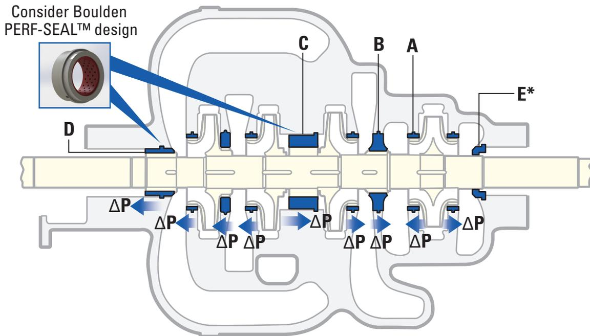
**A.** Case Wear Rings **B.** Inter-stage Rings **C.** Center Bushings **D.** Throttle Bushings **E.** Throat Bushings
