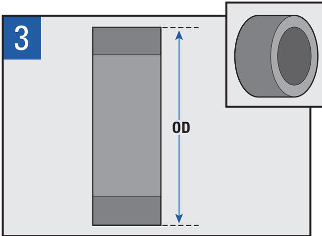
Calculate and machine part outside diameter.
