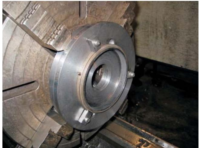
**Figure 3. Composite insert in metal case ring holder.**
