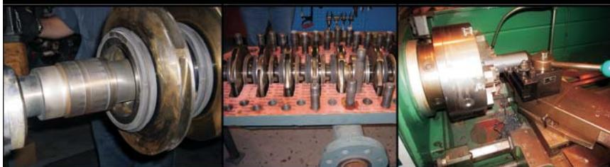
The Vespel® CR-6100 material is based on an advanced composite consisting of a high performance Teflon® PFA fluorocarbon resin and oriented carbon fibers. Wear components such as wear rings, throat bushings and line shaft bearings manufactured from Vespel® CR-6100 exhibit:
