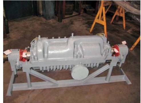
**Figure 1. The 9-stage boiler feed water pump.**
