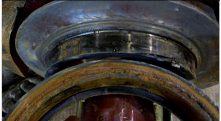
Figure 1 No-flow operation of a boiler feed water pump caused these metal wear rings to weld together, requiring extensive repairs. Replacement of metal parts with Vespel CR-6100 parts provided better operation in no-flow conditions.
