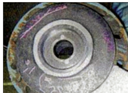
Figure 5 Replacing metal front and rear wear rings in a horizontal single-stage naphtha equivalent liquid transfer pump with Vespel CR-6100 parts enabled a major Asian pump manufacturer to reduce output power and increase efficiency
